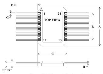
Figure III: Flatpack Package Detail
